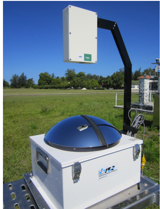
Figure 7 This Total Sky Imager belongs in ARM and sits in their Southern Great Plains Site. You can see the black bar on the mirror that covered the sun glare.
