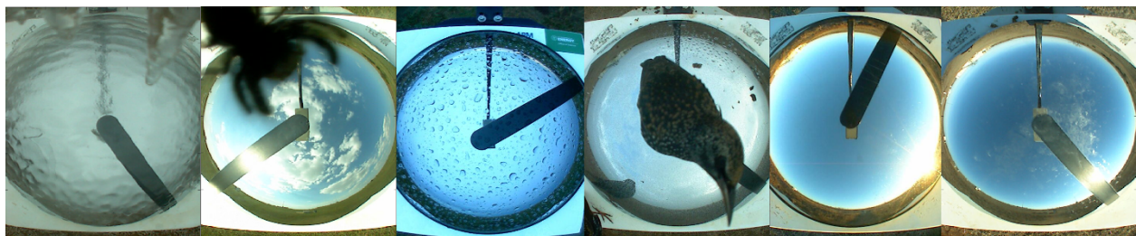
Figure 10 Some of the various "bloopers" images. a) If the weather gets cold enough, the mirror will ice over for days at a time and the camera housing will develop icicles, b) spiders and ants find home on the instrument. c) Rain is a common occurrence. d) Birds love the mirror which is also evidenced in the occasional fecal matter. e) Here the sun bar is completely askew from the sun, which is most likely a human error. f) Dirt and dust smeared on the mirror, resembling thin clouds.
