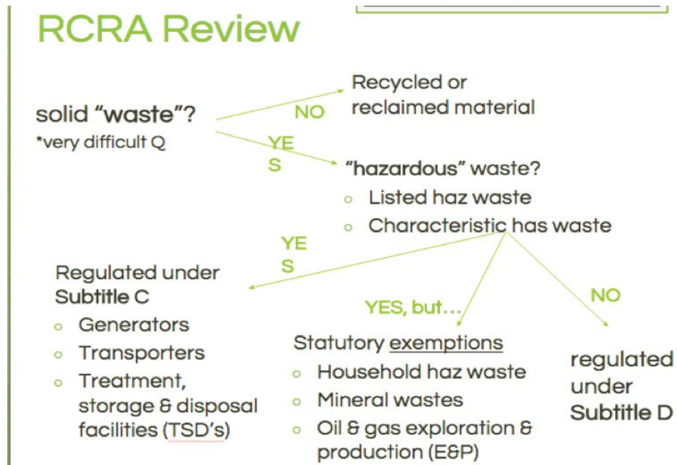
Figure 3. - This diagram shows the statutory definitions of solid waste, and hazardous waste and shows the the pathways of whether or not a waste is regulated by RCRA.
