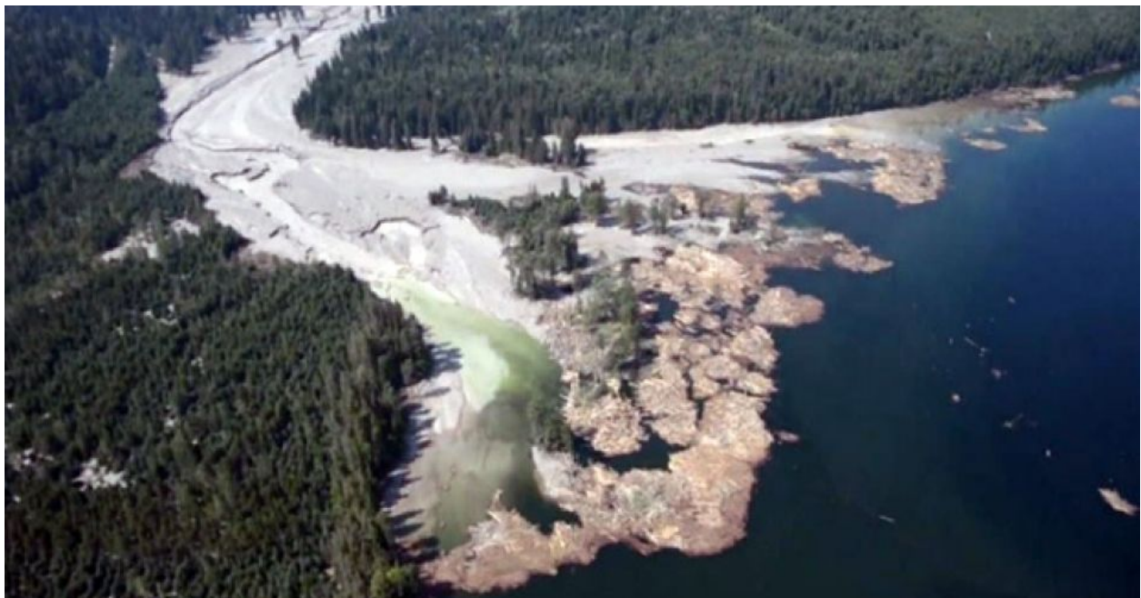
Figure 5: Mount Polley Mine Breach Aerial View (CBC Canada 2014).
