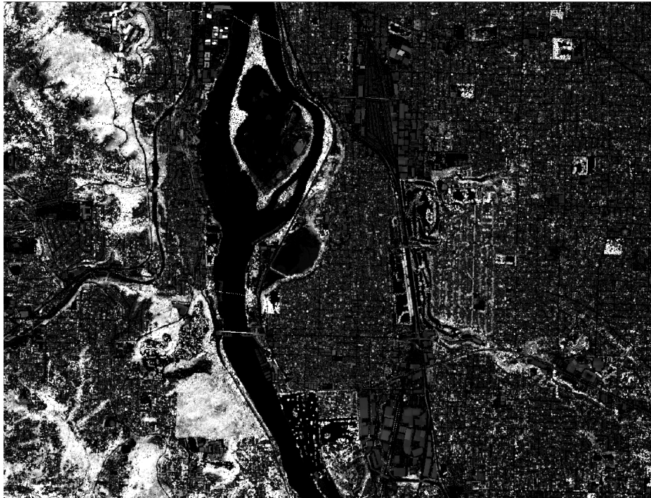
Figure 6: The raster image of Portland resulting from subtracting a terrain elevation lidar raster from a highest-hit lidar raster.
